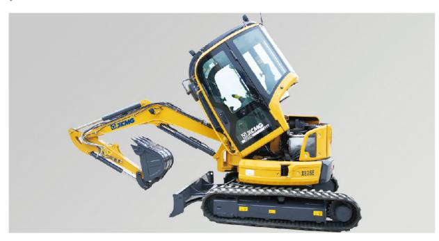
After the cab is tilted, the generator, start motor, muffler, electric and hydraulic systems can be maintained rapidly cooperated with fully-opened rear hood, there is no dead angle within 360 degrees for maintenance of whole machine.
